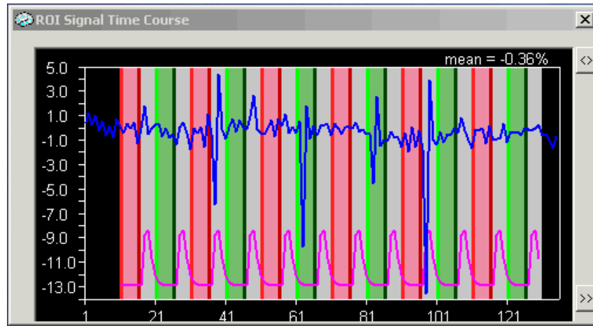
Spikes in signal, often due to abrupt head motion
